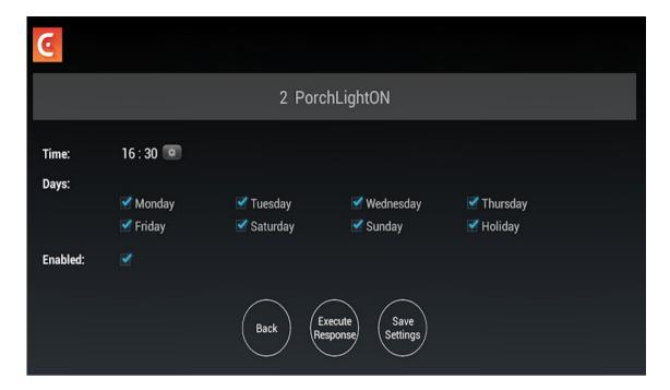
Select the Days of week for which the Schedule (Time Program) is enabled. The Time Program wil run at the Time indicated in the screen. This can be changed. Check the Enable Box to enable the Time program.
