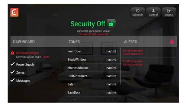
The centre pane shows the state of the security zones zonnected to the system; Active and Inactive. The right pane "Alerts" shows the list of events that have occured when the KT05 is online The top of the screen shows the Security Mode, ie "Security Off", "Away", "Night", "Day" To arm or disarm the system press the Security Mode Status button.
