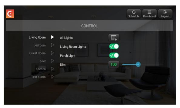
Up to 6 control groups are displayed. Each Control Group consists of Control Keys, and each Control Key consist of control actions.
