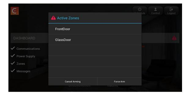
The options are to "Cancel Arming" (to abort the arming) and "Force Arm" (which means to automatically bypass all zones and arm the system).
