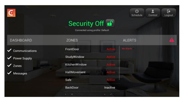
On the left is the alarm status summary, showing any Trouble alerts like Communications, Low battery Power Failure and Zone Trouble.
