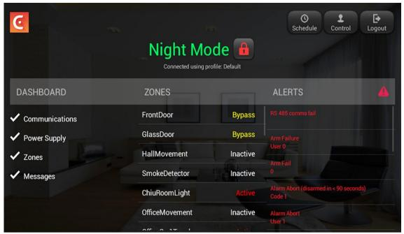
If any doors or windows have been bypassed as a result of Force-arming, the Bypass status is shown as above. Any open zones bypassed during force arming is automatically unbypased when the zone is closed.
