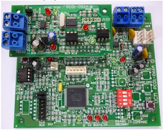
The UCM/Velbus is connected directly to the Velbus CAN bus.
