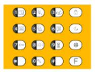
The bottom section has 16 buttons which correspond to the keypad buttons. When pointed at a keypad, the RC01 can be used just like a handheld keypad. The voice menu will be heard on the keypad. You can arm and disarm the security system as well as do anything that you could do with a Keypad. No programming is required for this function.
