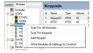
This will detect that KP04A is connected if all keypads have unique IDs. Select the KP04A on the left pane. The right pane shows the display below;
