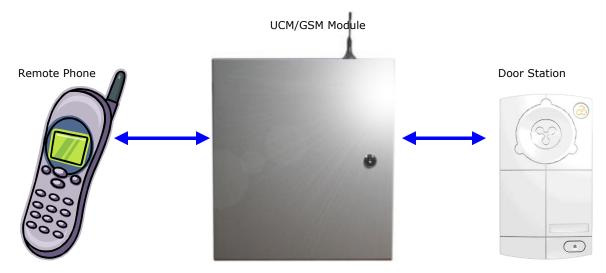
Note that this applies only when the intercom is between remote phone to Keypad/Door station via the GSM telephone number of the UCM/GSM.
